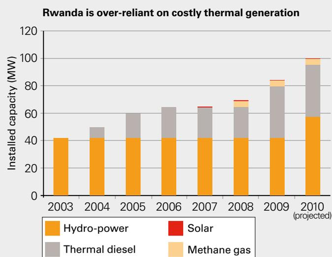
the government signed a contract for 15MW of rental diesel plant with AGGREKO, an independent power provider. Since then thermal power has increased from zero to its current level of 37.7MW – nearly half of Rwanda's generation capacity (Figure 3, above). The reliance on thermal generation with imported diesel fuel means that Rwanda is paying a great price to sustain its rapidly growing economy. It also means that economic growth is very fragile and threatened by the rising cost of oil.
